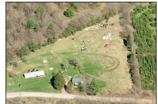
Above (top to bottom): Aerial view showing proximity of single-family home with large lawn and on-site septic system to nearby spring house; view of same house in context of springs and water tank; storage of junk vehicles on a property off of Bloomville Hill Road. Each of the land uses shown above are potential sources of spring water contamination and lay in the primary spring protection area as recommended by GEMS.
